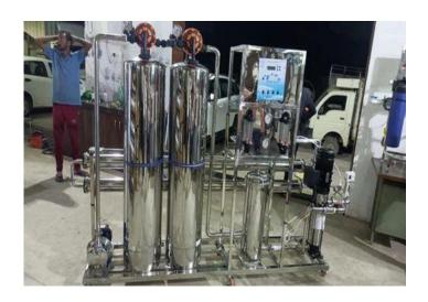
Keten Reverse Osmosis Water Purification Machine Capacity: 1000 liters/hr
